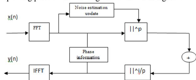
Figure 1 basic spectral subtraction method
