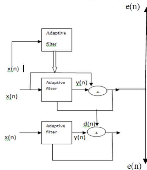
Fig.2. Classes of adaptive filters
